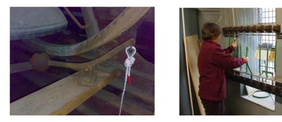
Fig. 6. An Ellacombe hammer and rack (here for 10 bells)
