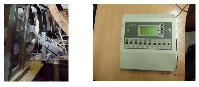
Fig. 7. An electro-magnetic hammer and a micro-processor controller
